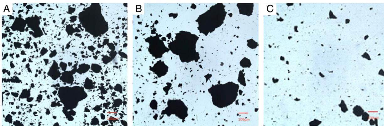
**Fig. 1.** Optical micrographs of the fragments produced from carbon black agglomerates infused with distilled water, processed at different temperatures: (A) 50 °C; (B) 80 °C; (C) 110 °C. Note the the scale bar depicts 100 μm.
