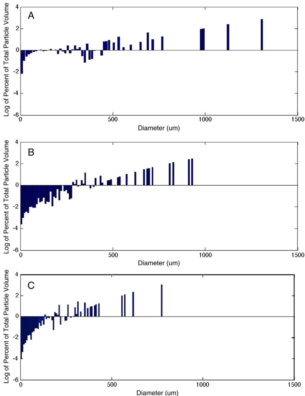
Fig. 2. Volume size distribution vs. fragment diameter for water-infused carbon black agglomerates processed at: (A) 50 °C; (B) 110 °C; (C) 150 °C. Note the decrease in frequency of large fragments at the elevated temperature.
