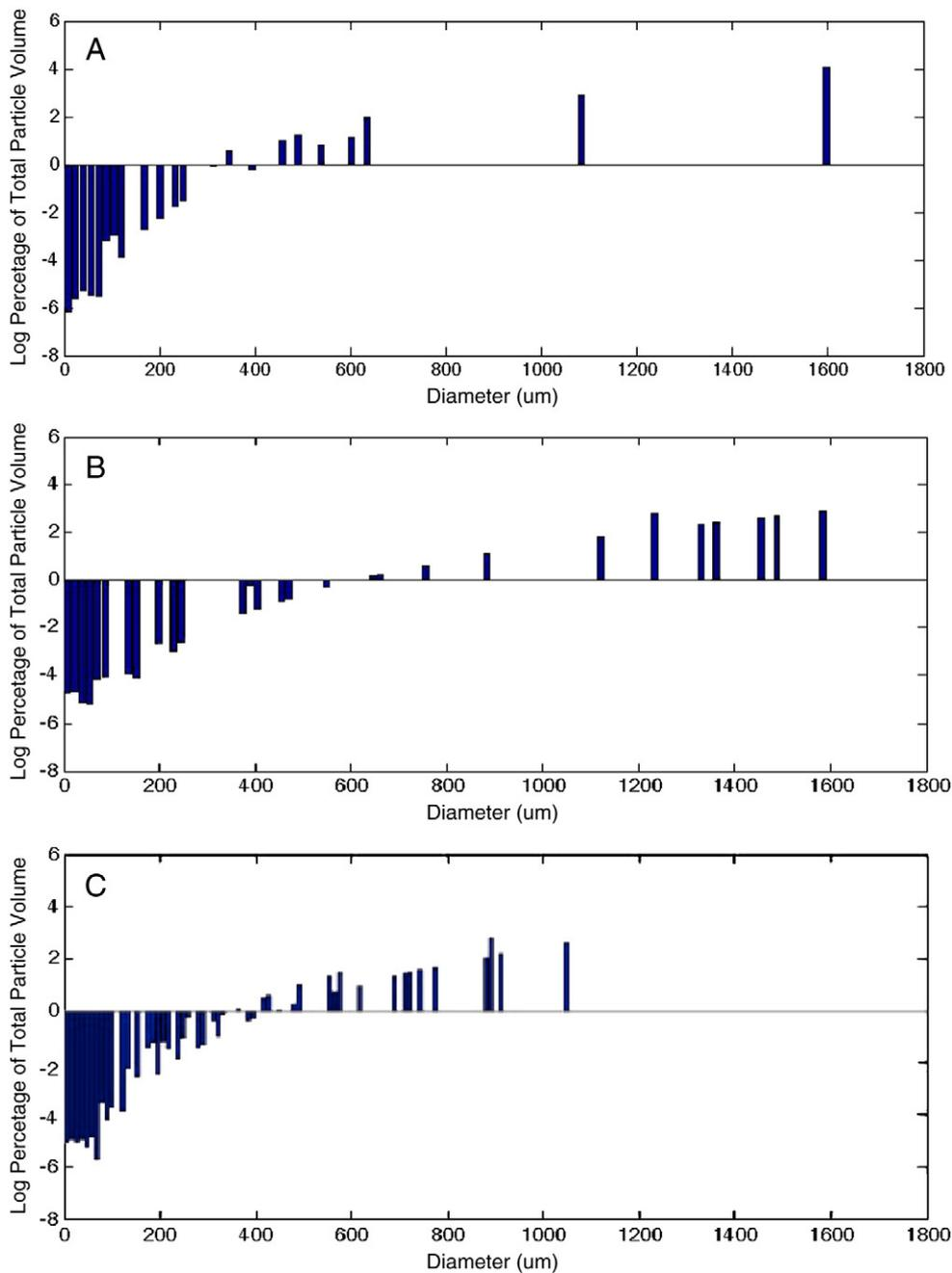
Fig. 3. Volume size distribution vs. fragment diameter for acetone-infused carbon black agglomerates processed at: (A) 45 °C; (B) 65 °C; (C) 85 °C.
