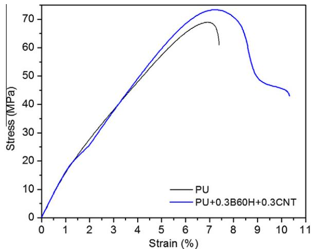
Fig. 1. Representative stress–strain curves for the neat polyurethane and the PU based composite containing 0.3 wt.% CNTs and 1x B60H.
