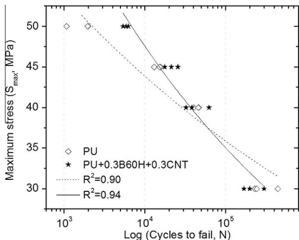
Fig. 2. S–N curves for the neat PU and PU/CNT composites.
