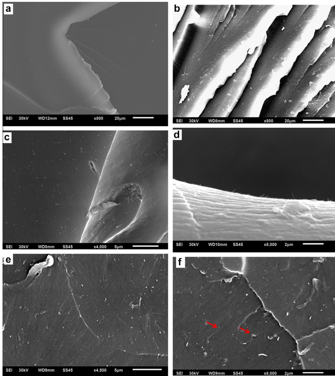
**Fig. 4.** Scanning electron micrographs of the fatigue fracture surface of the neat PU and composites: (a) neat PU,  $S_{\max} = 50$  MPa,  $N = 1962$ ; (b–d) composite,  $S_{\max} = 50$  MPa,  $N = 6245$ ; (e, f) Composite,  $S_{\max} = 30$  MPa,  $N = 167,921$ . The arrows in (f) pinpoint to individual CNTs bridging growing cracks.
