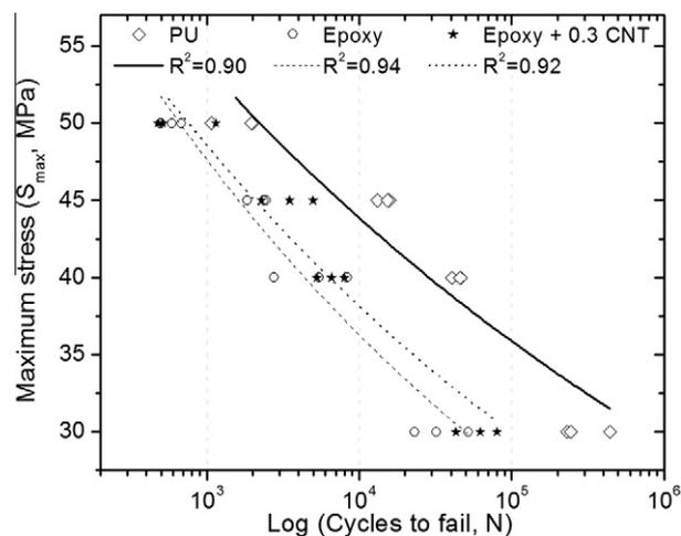
Fig. 3. Comparison between the S–N curves for the neat PU in tension–tension cyclic fatigue obtained in this study and the S–N curves for neat epoxy and epoxy reinforced with CNTs from Reference [13].
