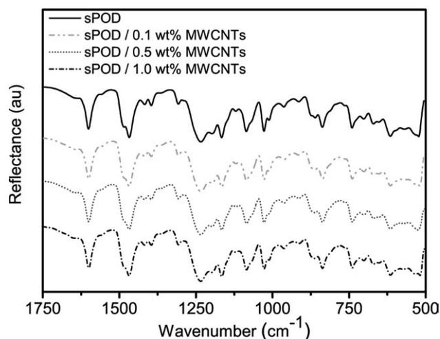
**FIGURE 2** Representative FTIR spectra of the neat polyoxadiazole and of the sPOD/MWCNTs composites.
