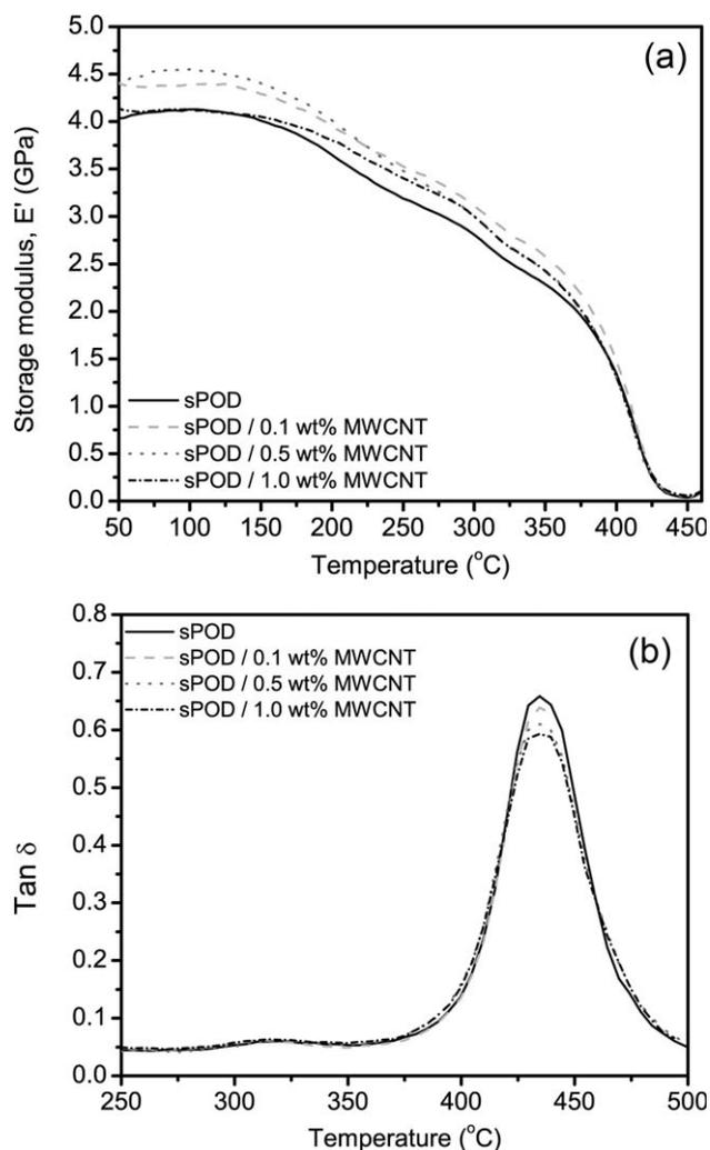
**FIGURE 8** Dynamic mechanical analysis of composites: (a) storage modulus ( $E'$ ) and (b)  $\tan \delta$  of composites reinforced with pristine MWCNTs.
