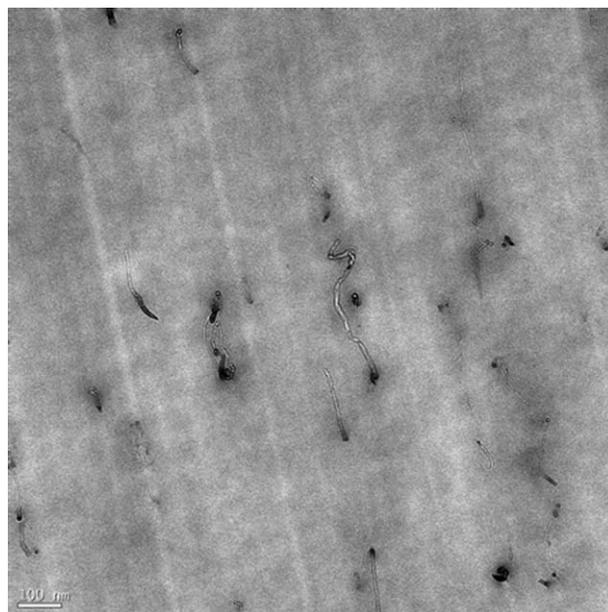
**FIGURE 5** TEM images of sPOD composite reinforced with  $0.5\text{ wt } \%$  MWCNTs.
