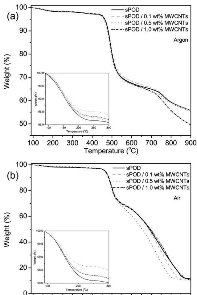
**FIGURE 9** TGA curves of neat sPOD and sPOD/MWCNTs composites measured under (a) flowing argon and (b) air flow.
