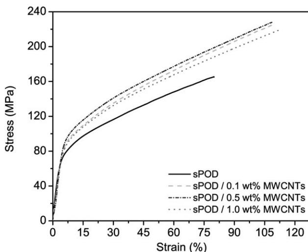
**FIGURE 6** Representative stress-strain curves for the neat polyoxadiazole and nanocomposites.
