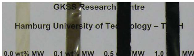
**FIGURE 4** Digital photographs of the neat polyoxadiazole and nanocomposites films reinforced with different amounts of MWCNTs.
