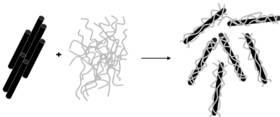
**FIGURE 3** Schematic drawing of the interaction between sPOD and pristine MWCNTs.
