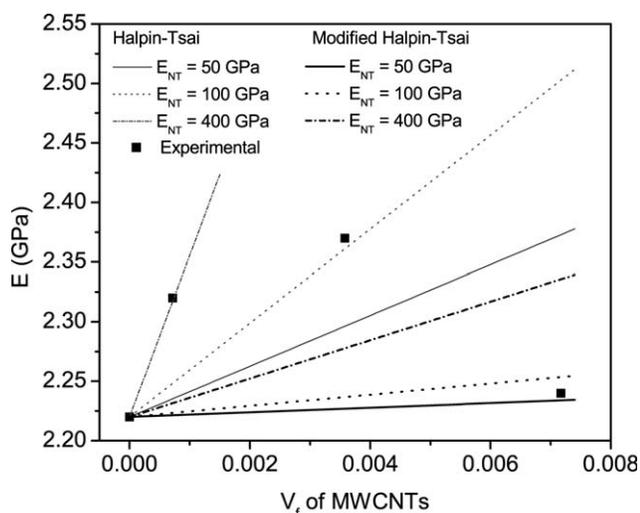
**FIGURE 7** Theoretical Halpin-Tsai and modified Halpin-Tsai models and experimental data for the sPOD/MWCNTs composites at various nanotube loadings.
