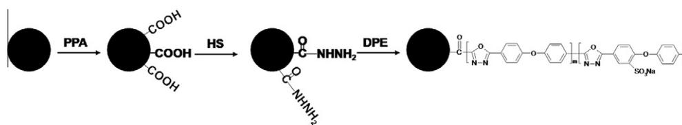
Fig. 1. Proposed route for the oxidation of the CB represented as a black circle and grafting of POD on its surface.
