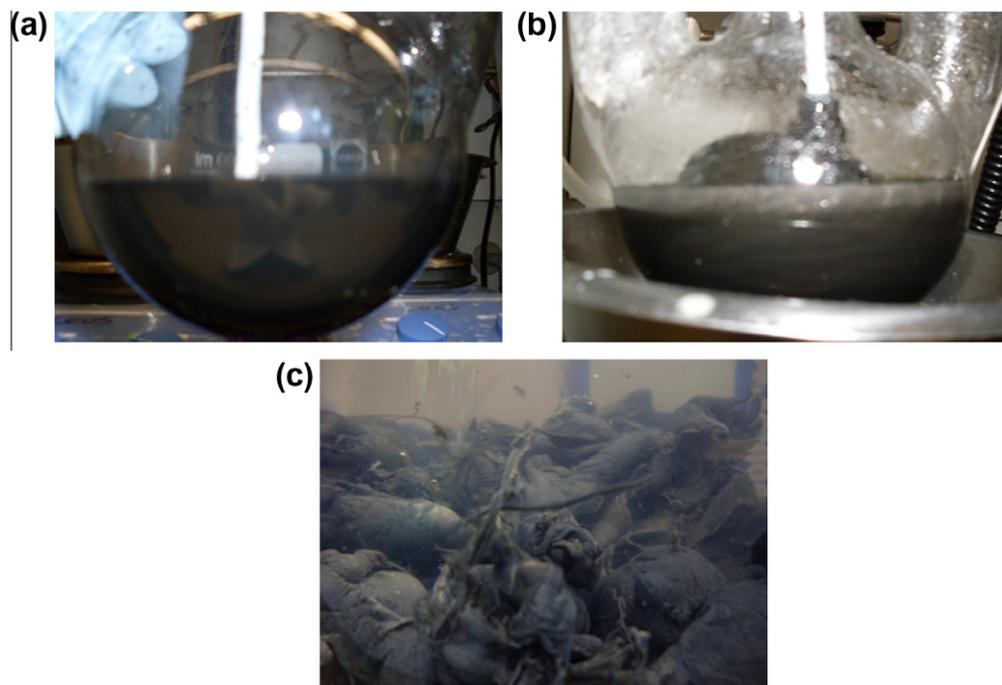
Fig. 2. Digital photographs of the reaction mixture: (a) after the pre-dispersion step, (b) 3 h after starting of the synthesis, and (c) composite precipitated like “noodles”.
