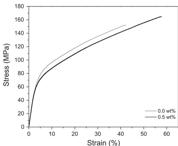
**Fig. 6.** Representative stress–strain curves of the CB/POD nanocomposites.
