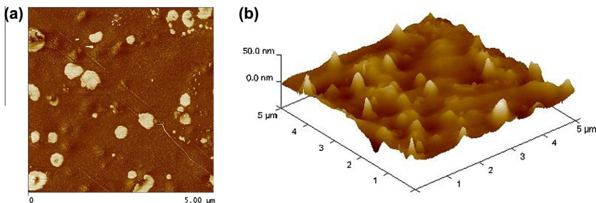
**Fig. 7.** AFM images of the fracture surface of the POD nanocomposites reinforced with 0.5 wt.% of CB after conducting tensile tests.
