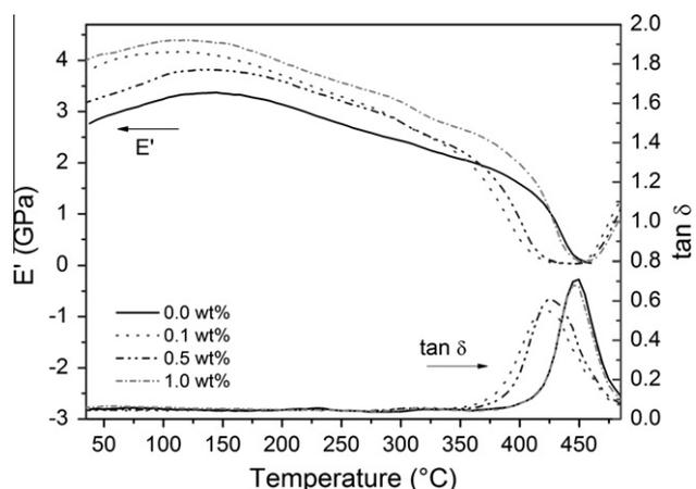
Fig. 5. (a) variation of the storage modulus ( $E'$ ) and  $\tan \delta$  as a function of temperature for the CB/POD nanocomposites.
