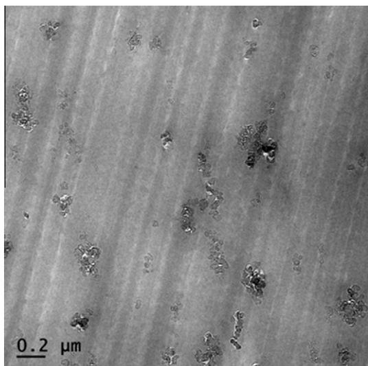
**Fig. 8.** TEM image of the fracture surface of the POD nanocomposites reinforced with 0.5 wt.% of CB after conducting tensile tests.
