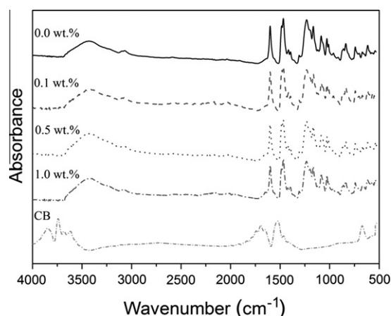
Fig. 4. Representative FTIR spectra of the neat polyoxadiazole, pristine CB and CB/POD composites.
