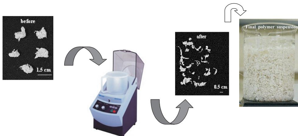
Figure 2. Polymer samples before and after of the shredder.
